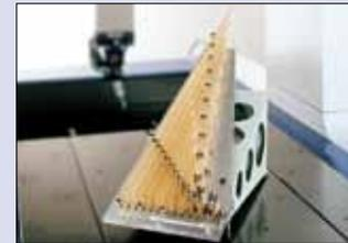
CMM calibration using a virtually zero thermal expansion glass gauge.
