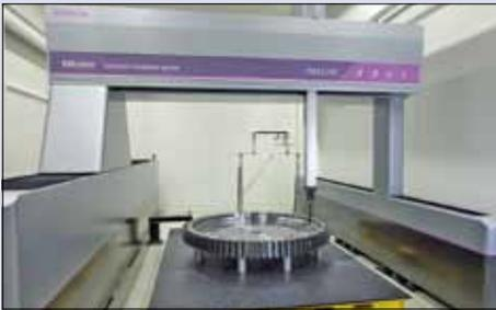
FALCIO-Apex 305020G measuring a gear for a wind turbine engine.
