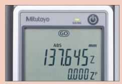
GO on the display and the panel LED showing GREEN means the measurement is within the tolerance limits.
