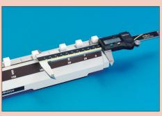
Checking the accuracy of a caliper (inside measurement).
