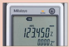
±NG on the screen and the panel LED showing ORANGE (-NG) or RED (+NG) means the measurement is outside the tolerance limits
