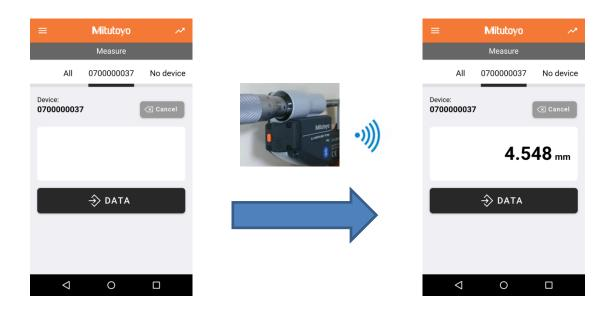
When multiple U-WAVE-TCB/U-WAVE-TMB are connected to the app, you can check the measurement values of all devices on the "All" screen. If no device is registered, "No connected device" is displayed.
