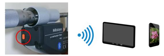
If the transmission is successful, the LED flashes green. The buzzer sounds twice for the buzzer type.
