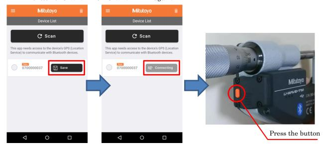
⑤ When the display of the application turns orange "Connected", the connection is completed.
